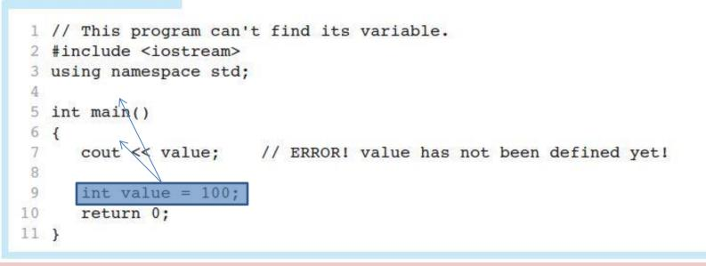
The program will not work because line 7 attempts to send the contents of the variable value to cout before the variable is defined. The compiler reads a program from top to bottom. If it encounters a statement that uses a variable before the variable is defined, an error will result.
