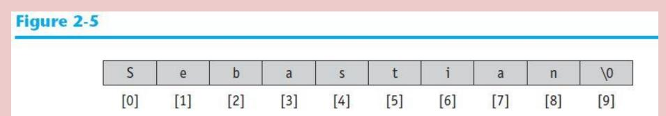
First, notice the quotation marks are not stored with the string. They are simply a way of marking the beginning and end of the string in your source code. Second, notice the very last byte of the string. It contains the null terminator, which is represented by the \0 character. The addition of this last byte means that although the string is 9 characters long, it occupies 10 bytes of memory.
