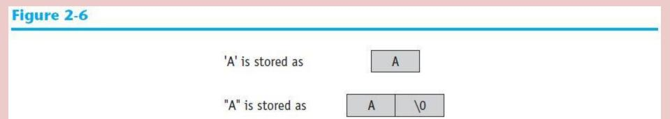
As you can see, 'A' is a 1-byte element and "A" is a 2byte element. Since characters are really stored as ASCII codes, Figure 2-7 shows what is actually being stored in memory.
